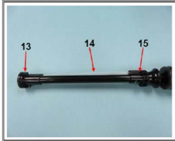
Figure 7: Shaft End, White Fabric Thread, and Black Plastic Runner (SGS 2018)
